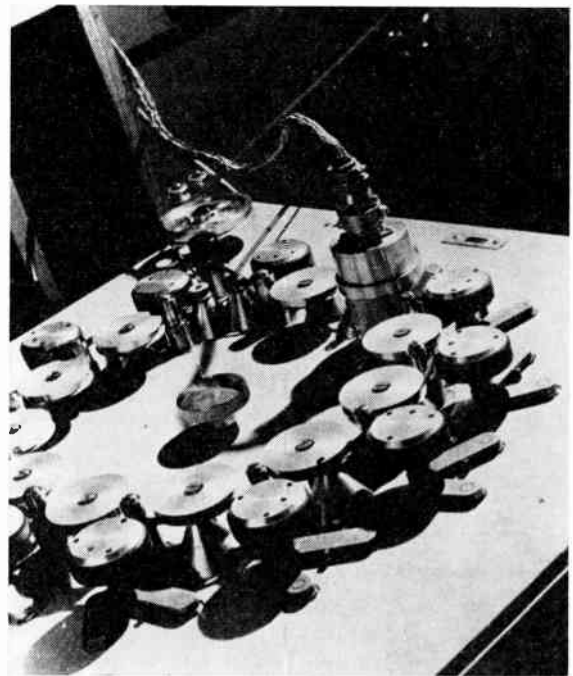
Fig. 19—The "Phonogène" of the Musique Concrète Group of the French Radio and Television System in Paris. A tape loop may be driven at twenty-four speeds using a keyboard control which is not shown. (Photograph courtesy of UNESCO.)
