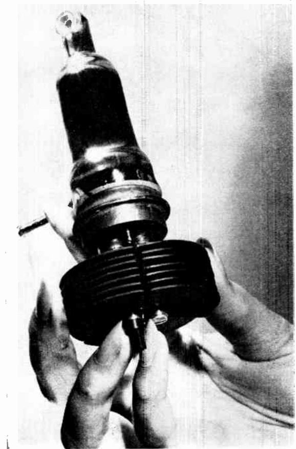
Fig. 6—Two-stage photocell microrefrigerator.
