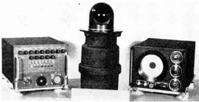
Fig. 7—Airborne infrared scanner, and associated electronics.
