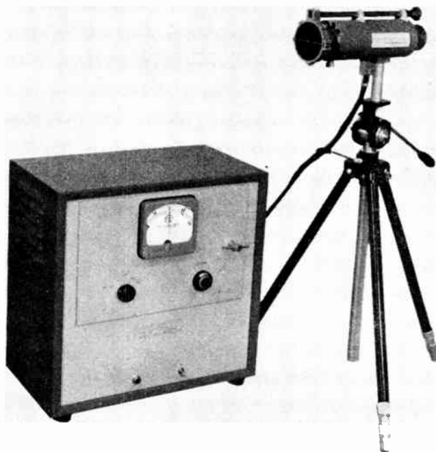
Fig. 5—Servotherm pyrometer model 1372.
