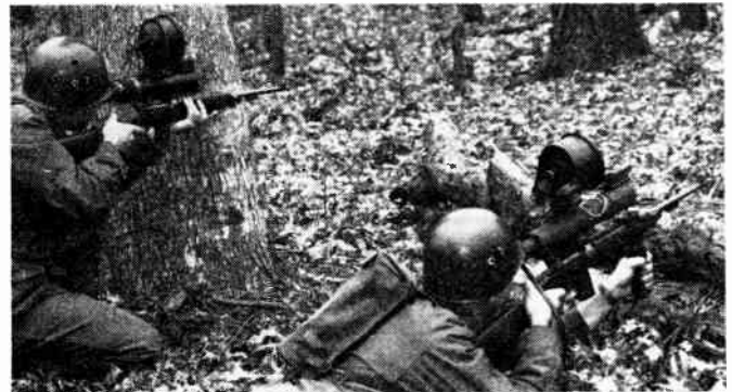
Fig. 2—Sniperscopes mounted on carbines for use by foot soldiers.
