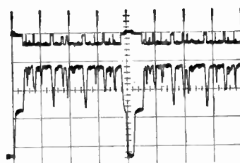
Fig. 10—Sync amplification and stretching. Top—input; bottom—output; scale—20 v/cm.
