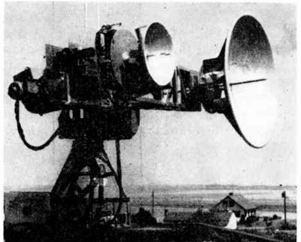
Fig. 1—Microwave antenna assembly (4-foot parabola—3 cm; 18-inch parabola—8 mm) at Ipswich, Mass.
