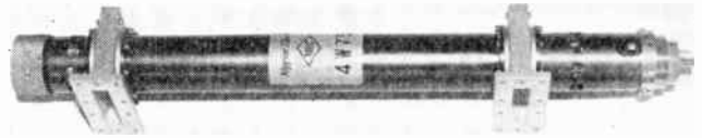
Fig. 16—Package type traveling-wave tube (type 4W75), used for improved repeater shown in Fig. 15.
