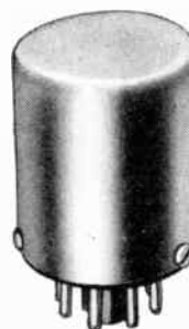
JK-G4: "Glasline" Crystal Filter Resonator. For broad filter applications, such as power line carrier communications and telemetering. Frequency range 50 to 200 kc.
