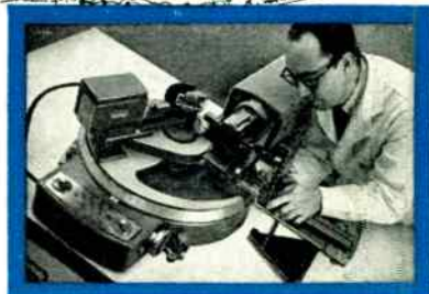
X-ray diffraction orients crystals prior to slicing wafer for silicon junction diodes.
