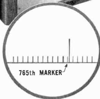
Observed pulse as viewed on a suitable synchroscope (magnification: 1000 to 1)
