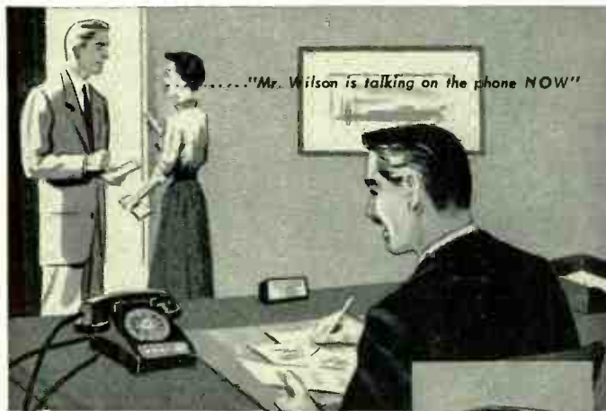
"HANDS-FREE" TALKING. Telephone set base has a built-in microphone — you talk without picking up handset. Tiny desk speaker amplifies the distant voice so that several persons in a group can listen to the conversation. For privacy, you lift the receiver, automatically shutting off the microphone and speaker. Small amplifier, not visible in the picture, furnishes power.
