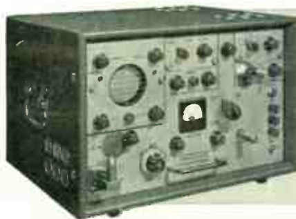
Kearfott X-band Test Set, frequency range 8,500 to 10,000 MC; a unique all-purpose portable radar test set, comprising a power monitor, spectrum analyzer, wave-meter and signal generator which supplies an accurately calibrated signal of known level with variable amplitude and pulse-width combinations. Also provides FM, square wave and CW output.
