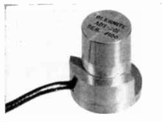
Glennite Model ADT-701 Accelerometer Specifications: Range, \pm 1 g; Sensitivity with 400 cps carrier, 125 mv per g/volt input; Maximum input voltage, 10 v r.m.s.; Size, 1\frac{1}{2} " d x 2" h; Weight, 3 oz.
