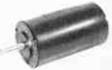
E Frame—Totally enclosed induction motor. 400 cycle 2, 4, 6 or 8 poles. 60 cycle 2 or 4 poles. 2-5/16" dia. H.P. up to 1/25 (up to 1/10 H.P. for axial vane blower application.)
