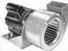
631 x 35—115 Volt, 60 cycle or 220 Volt, 60 cycle, 1 or 3 phase. 3450 RPM continuous duty. 250 CFM at 2 1/2" water gauge. Used in microwave generators, unattended repeater stations. Fits in space 13 1/2" long, 8 3/4" wide, 7 3/4" high.
