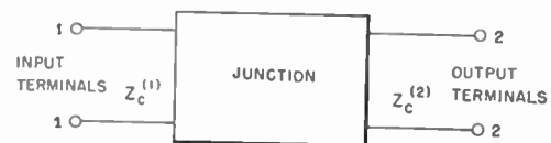
Fig. 1—Equivalent network representation of a two-port waveguide junction.
