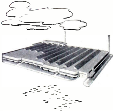
Rubber model for studying electron optical designing—basis for Rauland's exclusive Indicator Ion Trap.
