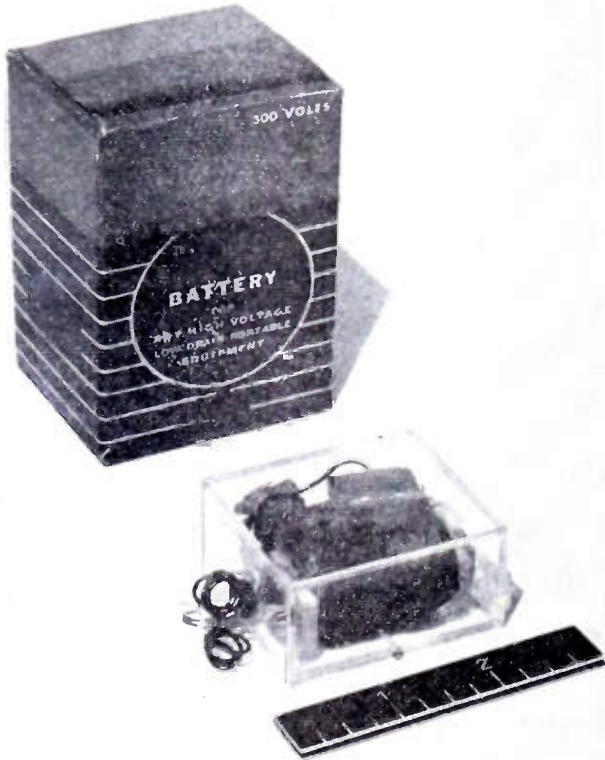
Fig. 3—Shows relative size of 500-volt transistor power supply as compared to a 300-volt battery.
