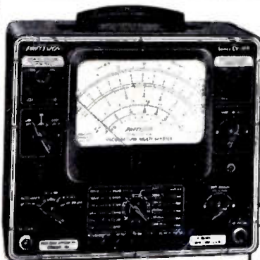
SERIES EV-10A True Zero-Center VTVM and Multi-Range Test Set with Direct Peak Reading High Frequency Scales.
