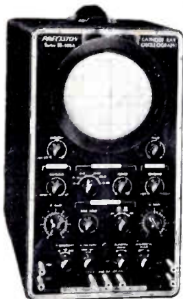
SERIES ES-500A High Sensitivity, Wide-Range 5" OSCILLOSCOPE 20 MV per inch "V" Sensitivity
