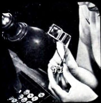
Completed mounts are inspected for visual defects.
