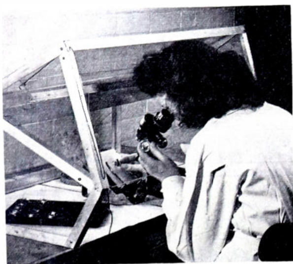
Fig. 12—Inspection position for trustworthy valves. Operator looks into microscope through a glass panel.
