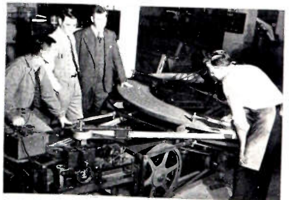
Seven miles of Revere copper bus bar were wound into great coils for the cyclotron electromagnet. The University built the winding machine itself, and wound the coils in its own shop. The special Revere bar is soft temper, free from scale, with rounded edges.
