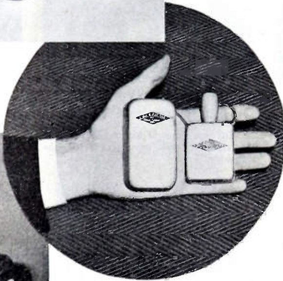
Above—A short range FM transmitter (right) with battery (left) which can be hidden in the pocket allowing a performer complete freedom of motion during a lecture.
