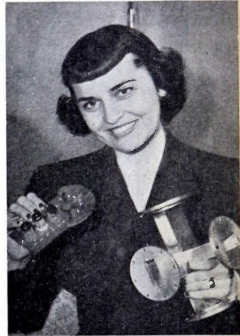
Above, right—A conventional bulky waveguide (right) is compared with the same component produced by Federal's new microwave wiring technique employing printed circuits.
