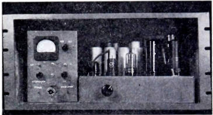
Fig. 5—Heterodyne type aural monitor.
