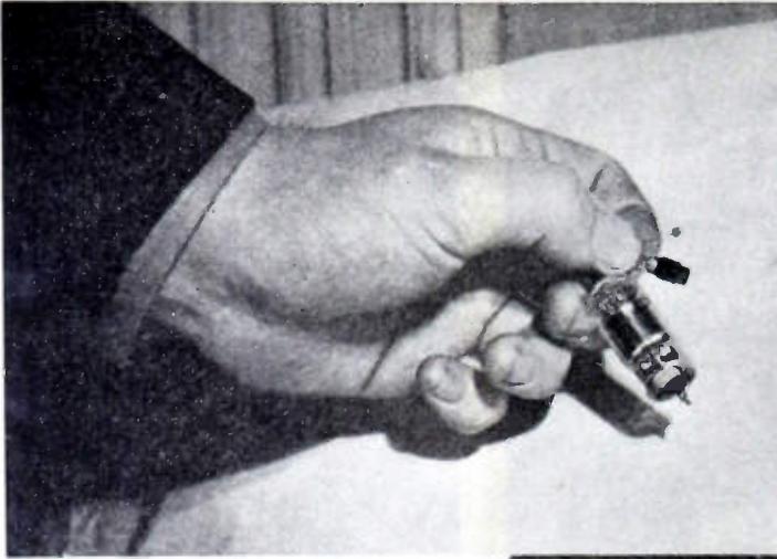
Above—Pea-sized transistor, dramatic new development in electronics, shown with its case (middle, compared with subminiature tube which it replaces in Signal Corps equipment.
