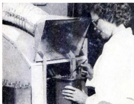
Transformer covers are press-fitted to case for strength, then solder-sealed against dust and moisture on this induction heater.
