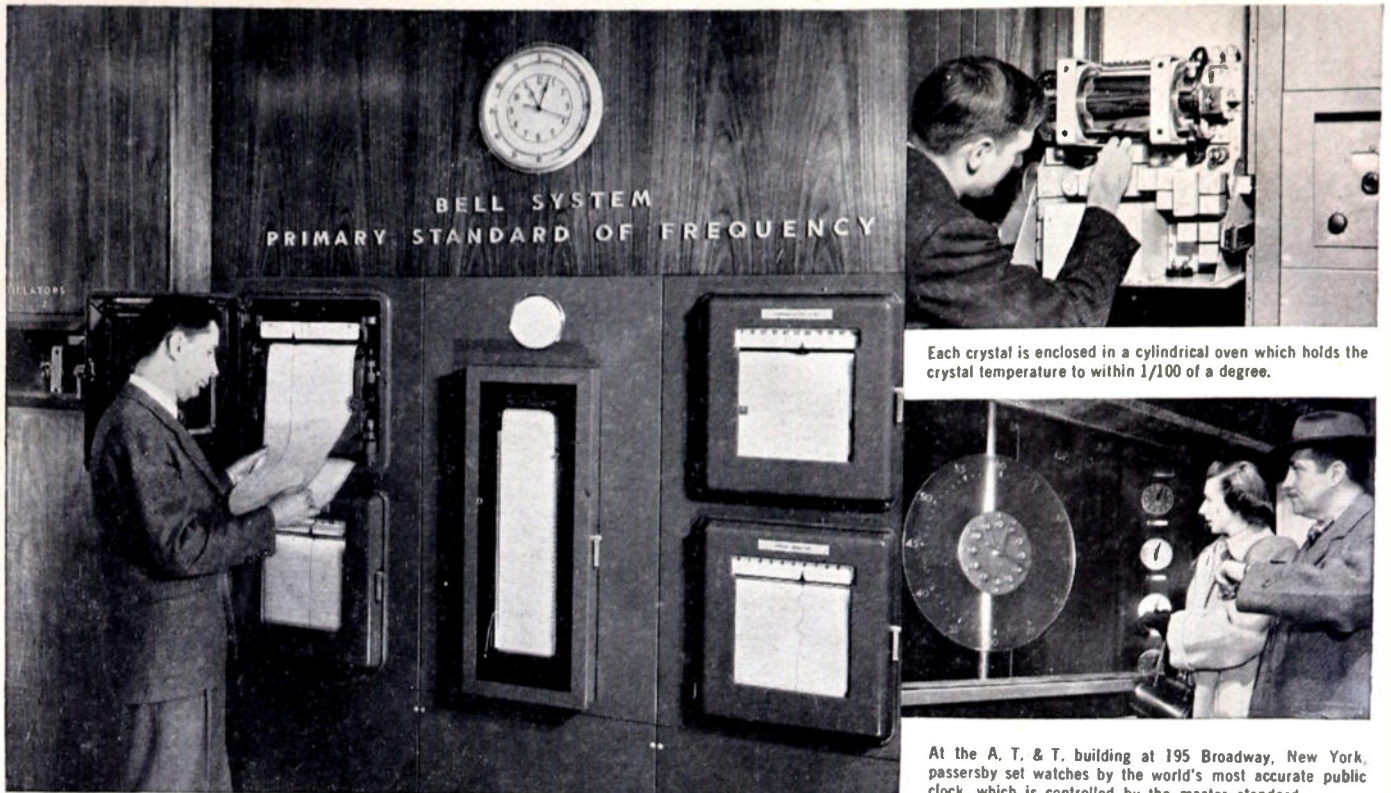
▲ Front of the new frequency-time standard at Bell Telephone Laboratories. In the rear there are 600 electron tubes and 25,000 soldered connections. Room temperature is maintained within two degrees.
