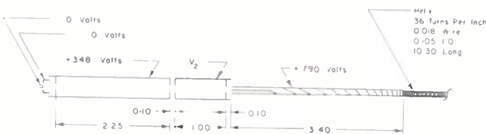
Fig. 8—Tube No. 112. Beam current 0.60 ma. Dimensions in inches. These are the important dimensions and operating conditions of an experimental low-noise tube for which the theoretical and experimental noise figures are compared. This tube employed the spiral-type rf input and the double-velocity jump noise-reduction configuration.
