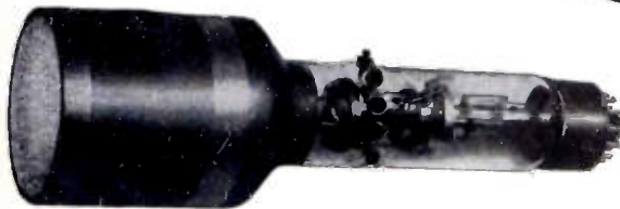
TYPE K1065P — 3-inch flat-faced tube with high deflection sensitivity. Deflection-electrode connections through neck enable high-frequency applications.
