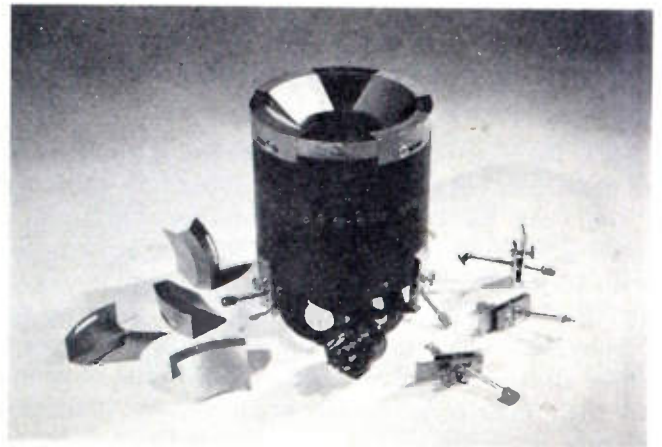
Fig. 5—Section-wound yoke for 45^\circ deflection, complete with compensating trimming tabs and beam alignment magnets.
