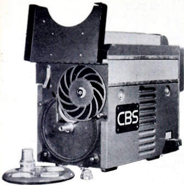
Fig. 20—RCA monochrome camera converted for color, front view; lens turret removed and added color disk in place.
