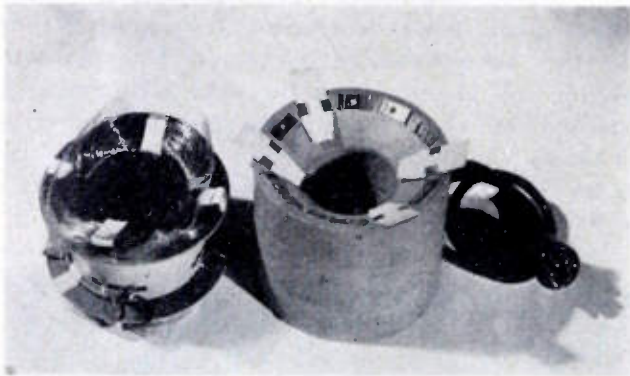
Fig. 11—At left is the unmounted 45° multi-beam deflection yoke, adapted for machine winding and die forming. The completed yoke, in its case, is shown with four compensating tabs in their approximate operating arrangement, at right.
