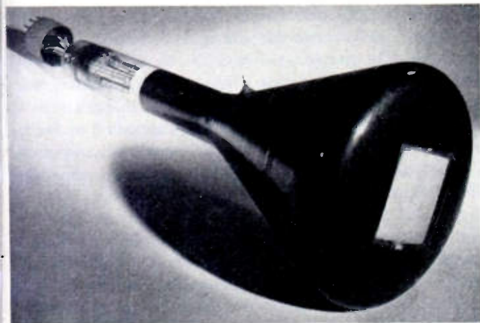
Fig. 8—Experimental shadow-mask color tube containing a test sample of dot screen.
