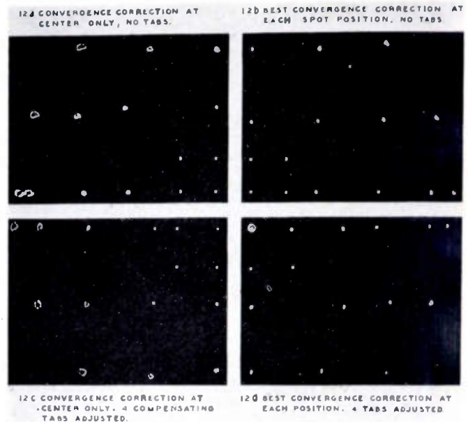
Fig. 12—Spot patterns using formed-winding yoke of Fig. 11, with 45° maximum deflection angle. (The circle around the axial dot in 12 (d) indicates the required dynamic convergence amplitude.) (a) Upper left quadrant, convergence correction at center only, no tabs. (b) Upper right quadrant, best convergence correction at each spot position, no tabs. (c) Lower left quadrant, convergence correction at center only, 4 compensating tabs adjusted. (d) Lower right quadrant, best convergence correction at each position, 4 tabs adjusted (final result).
