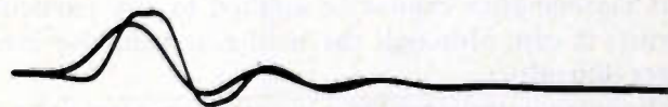
Fig. 14—Normal and crispended \frac{1}{4} -microsecond pulse waveforms for a system of 2-mc bandwidth to the 3-db point.
