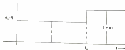
Fig. 2—Unit step function at time zero followed by a step function of depth m at time t_0 .
