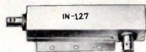
Aerovox Type IN-127 mounted inside voltage regulator (Arrow No. 1) and acting as interference eliminator for voltage regulator and generator systems.
