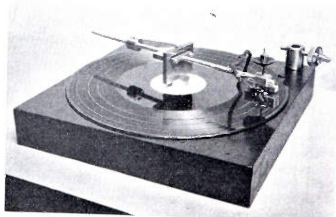
Fig. 5—This shows the pickup arrangement used to measure the amplitude of cut of the recorded groove. Amplitudes as low as 25 microinches were readily measured.
