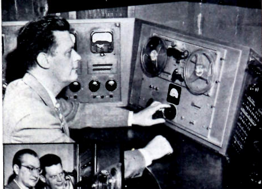
PT6-A Magnecorder and amplifier in rack mount. WGAR, Cleveland
