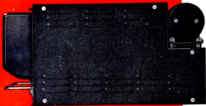
51V-1 glideslope receiver, covers in place
