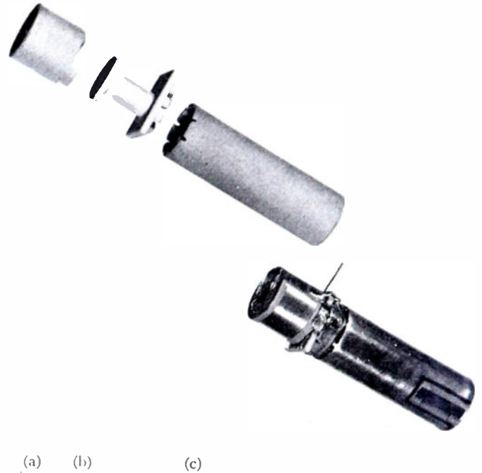
Fig. 4—Model PC-IV, printed intermediate-frequency amplifier design based on unit construction of a single-stage unit. Unit printed assembly contains subminiature electron tube and principal circuit components associated with each stage, including inductor assembly. Three basic parts form the stage unit: (a) high-K ceramic tube, (b) steatite inductor form, and (c) high-K ceramic tube.
