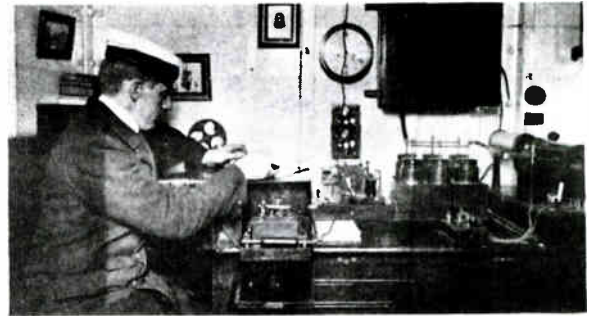
Marconi spark installation on S.S. Minnehaha , 1904. Note tape, coherer, 10-inch coil and the tuning coil in aerial.
