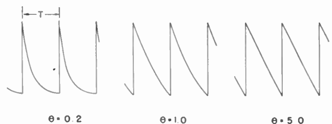
Fig. 4—Calculated wave forms for e_C in a series RC circuit.
