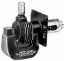
Raytheon magnetron used in the "Microtherm," the microwave diathermy equipment.
