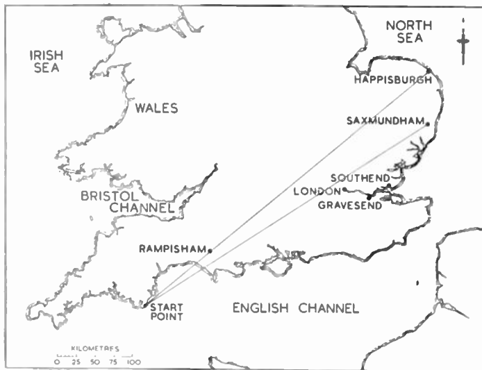
Fig. 3—With a transmitter erected at Start Point, field-strength measurements were made at many points on a line with Happisburgh and Saxmundham.
