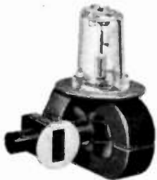
One of the Raytheon magnetrons used in airborne radar apparatus.
