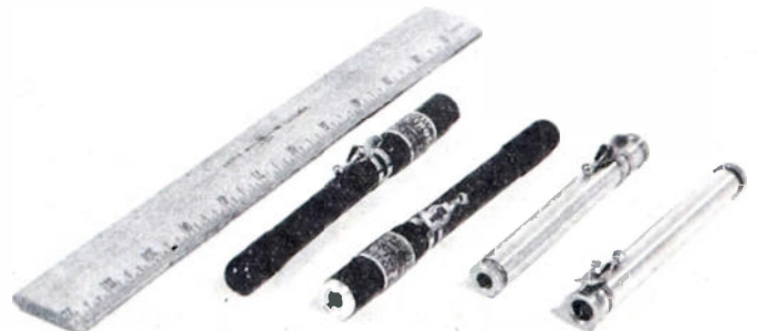
Fig. 9—Pen-sized fiber electroscopes or dosimeters for use in high-level radiation areas.
