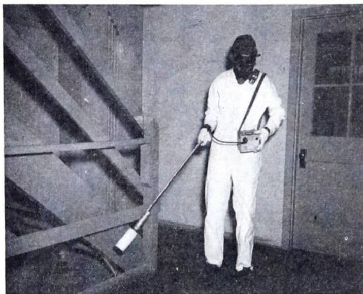
Fig. 21—Fish-pole meter for measuring high levels of radiation.
