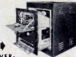
CONTROL UNIT — Operates as an electronic repeater in teletype lines.
