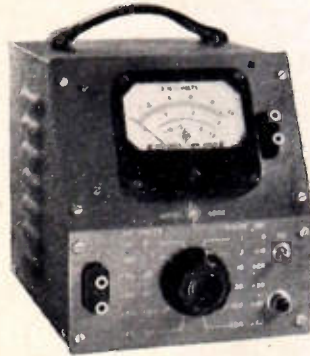
-hp- 400C Vacuum Tube Voltmeter Wide range, 20 cps to 2 mc, 12 ranges, 0.001 v to 300 v, flat response, 10 megohms input impedance.
