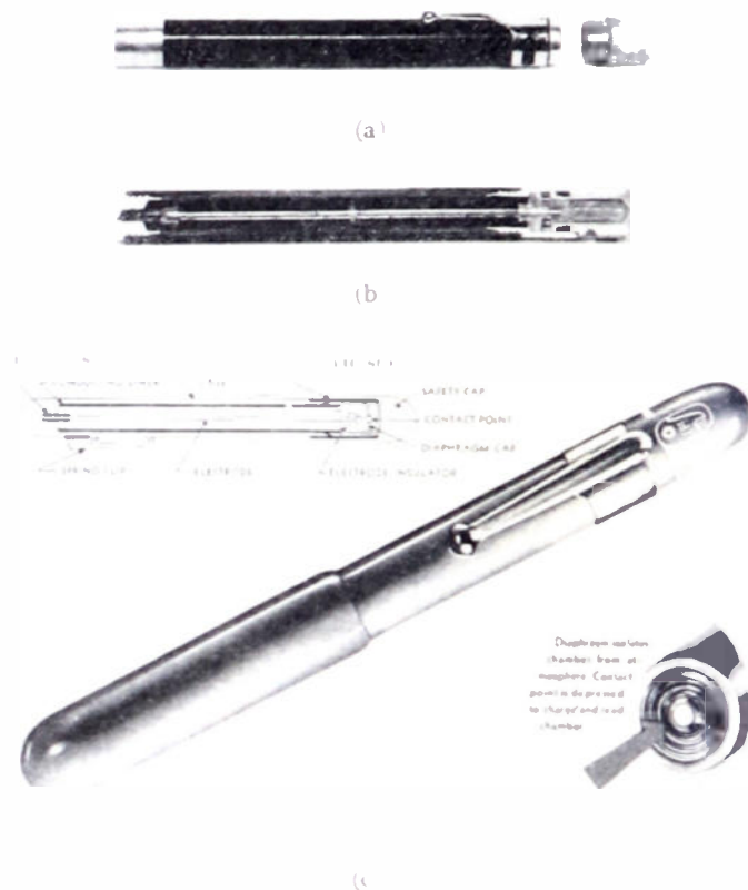
Fig. 1—Pocket meters worn in areas where radiation exposure is possible. (a) Type used originally at Oak Ridge National Laboratory. (b) Improved meter of type (a). (c) Rose pocket type.
