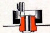
Silicone bushings and plastic cups used with capacitors 660-v a-c, or 1500-v d-c and lower.
