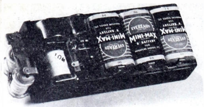
Fig. 10—Electronic pocket meter complete with batteries.
