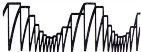
Fig. 19—Conversion of sawtooth to step function.
