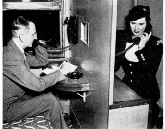
Fig. 8—Telephone facilities installed on train.
