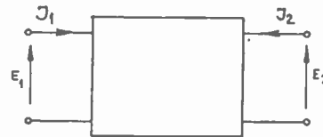
Fig. 10—Schematic diagram of a four-terminal network.
