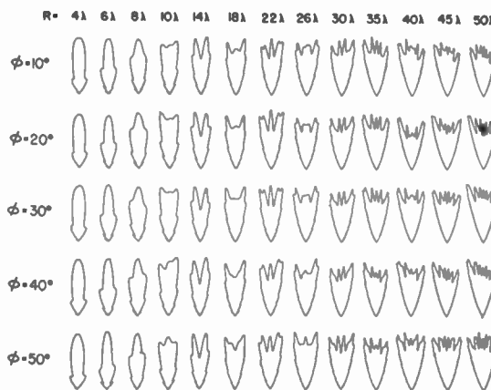
Fig. 2—Comparison of E -plane patterns for a horn having a constant flare angle in the E plane but a variable H -plane flare angle.
