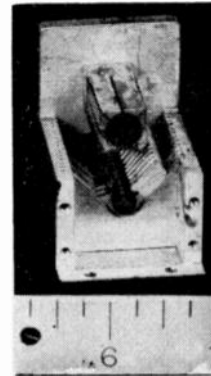
Fig. 7—A concentric distributed-capacitance line by fringe effect.
