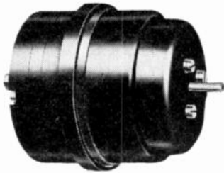
INDUCTION GENERATOR: when fed from AC source produces voltage proportional to speed of rotation. Used in circuits as velocity control component.
