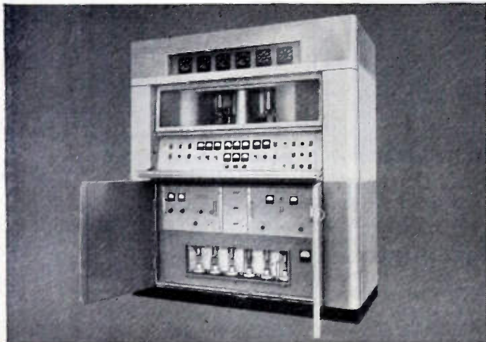
CENTRALIZED CONTROLS... all major controls are located on the front panel to make simultaneous adjustments easy. All tubes are replaceable from the front of the cubicle.
