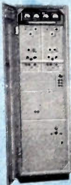
RADIO TRANSMITTER 186-A. Provides maximum operation on 1 phone channel and 1 CW channel simultaneously, or 2 CW channels simultaneously, with choice of 2 frequencies.
