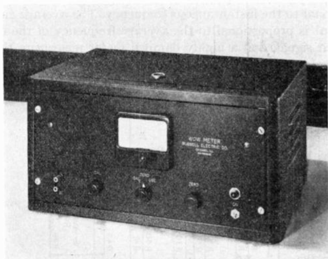
Fig. 1—Front view of the wow meter.
