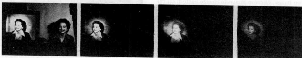
Fig. 10—Comparison of sensitivities of image orthicon and 35-millimeter Super XX film. (Incandescent light source.) (a) 2 foot-lamberts (b) 0.2 foot-lambert (c) 0.07 foot-lambert (d) 0.02 foot-lambert
