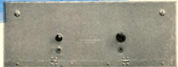
Front view, showing panel in operating position. Hinged at the bottom, this panel, when open, allows voltage measurements and inspection of all components to be made while set is operating, without removing it from the rack.
