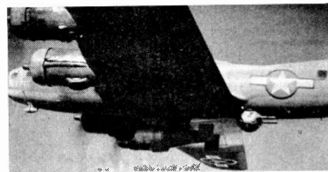
Fig. 58—B-17 airplane with one GB-4 glide bomb suspended on an external bomb rack.
