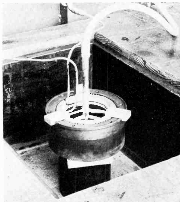
Fig. 15—Internal-gear-tooth hardening at 450 kilocycles.
