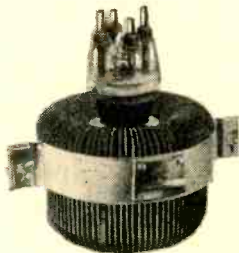
AmpereX Type 889-R Transmitting Tube. Filament voltage, 11 volts. Filament current, 125 amperes. Amplification factor, 21. Direct interelectrode capacitance: grid to plate, 20.7 \mu\text{f} ; grid to filament, 19.5 \mu\text{f} ; plate to filament, 2.5 \mu\text{f} . List price, $325.00.
