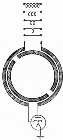
Fig. 30—Schematic diagram of range switching in a cylinder circuit.
