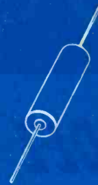
One use of "SF" Type Powder is in high frequency choke cores (with sealed-in leads).
