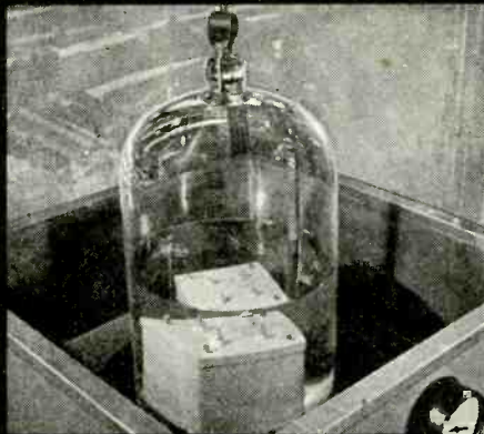
IMMERSION VACUUM TEST of each unit—not just random units—after final assembly, is standard procedure at AmerTran. Quality control of hermetic sealing is thus rigidly maintained.
