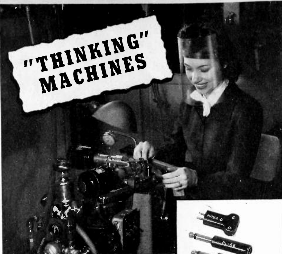
Machine designed by Remler to perform multiple operations: automatic slotting; indexing; drilling; milling and reaming.
