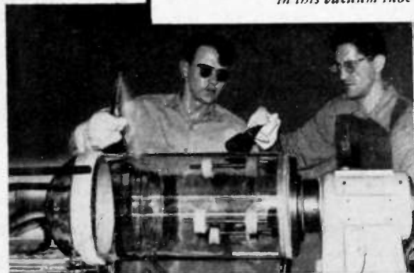
Making very large glass seals requires expert handling. Two 17" glass cylinders are being joined
