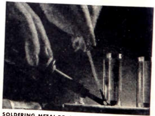
SOLDERING METAL TO GLASS is one of the things they said "couldn't be done". . . but many companies are now doing it every day. With Corning's method the base for the solder becomes part of the glass itself, providing a permanent hermetic seal.
