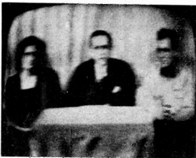
Fig. 16—Example of smear ghost. Picture as received 45 miles from transmitter with 1600-foot hill between receiver and transmitter.
