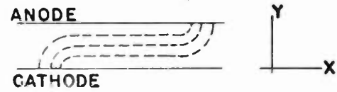
Fig. 16—Electronic trajectories in a plane magnetron.
