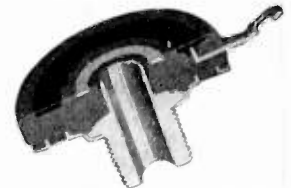
Cross section of Bradleyometer showing how terminals are imbedded in solid, molded resistor. (Actual size.)
