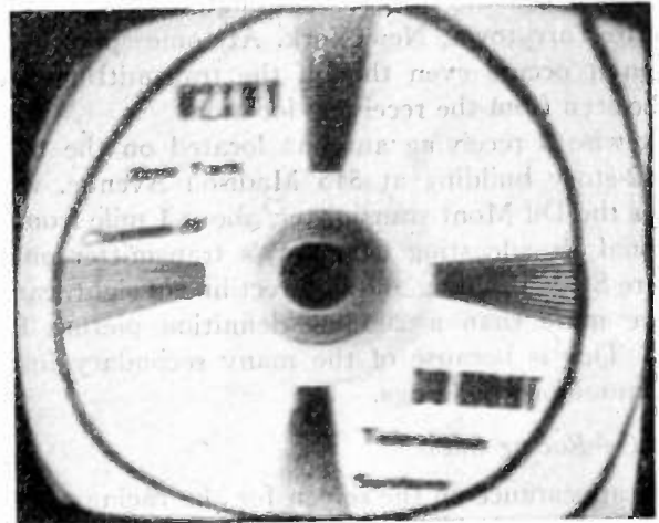
Fig. 15—Example of smear ghost. Test pattern as received 45 miles from transmitter with 1600-foot hill between receiver and transmitter.
