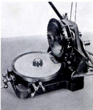
This printing machine has been developed by G-R to print scale calibrations on a six-inch dial which is hand-marked at over 1,500 points on a scale with an effective length of 15 feet.
