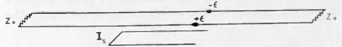
Fig. 18—Auxiliary arrangement in which generator E is in series with the short-circuiting bar.
