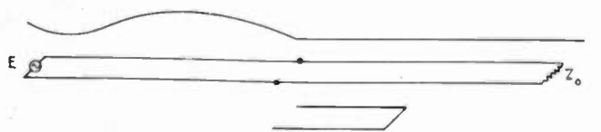
Fig. 15—Current distribution in a transmission line with a coupled section when X > 0 . The standing wave starts above the open ends of the section.
