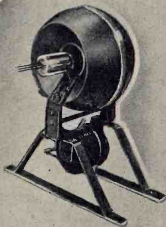
● A developmental r-f amplifier stage using the RCA-825 at 500 Mc. The photograph shows the resonator, the tube, the electromagnet and general arrangement of parts. In use at RCA Communications, Rocky Point, Long Island, N. Y.
