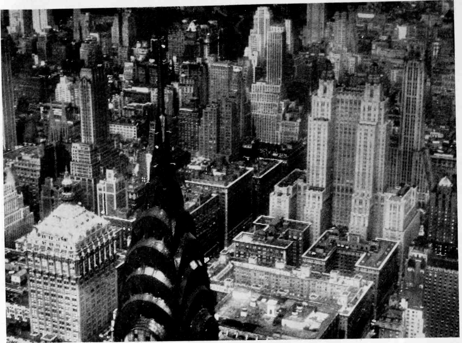
Fig. 14—Scanned reproduction of Fig. 13 (441 lines, 30 frames, 4.25 megacycles, slit aperture).
