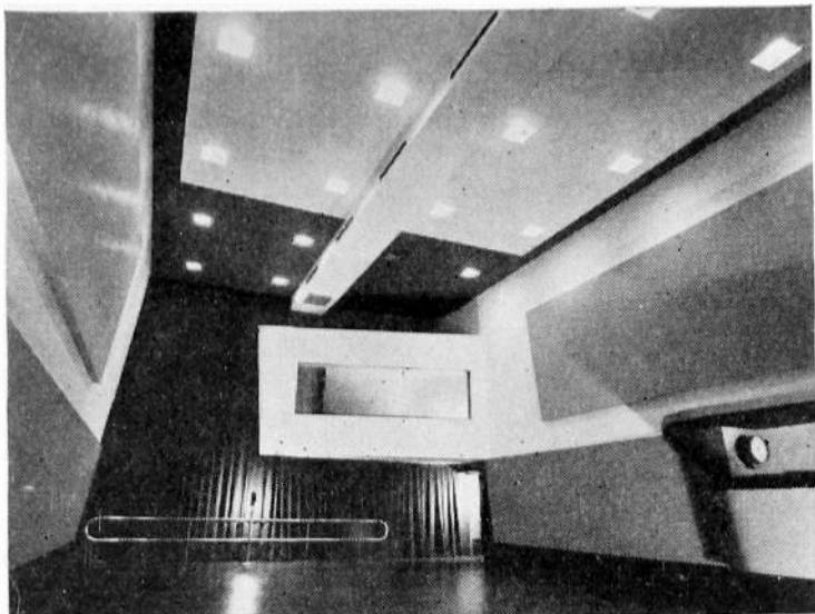
Fig. 5—A view from the microphone end of KNX Studio 2 showing the observation room and the new sloping-wall treatment.
