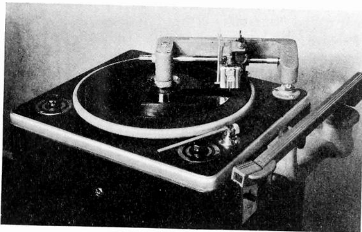
Fig. 1—Recording and reproducing equipment for broadcast use.
