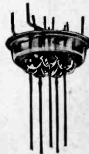
View of moulded glass stem assembly showing individual lead seals.
