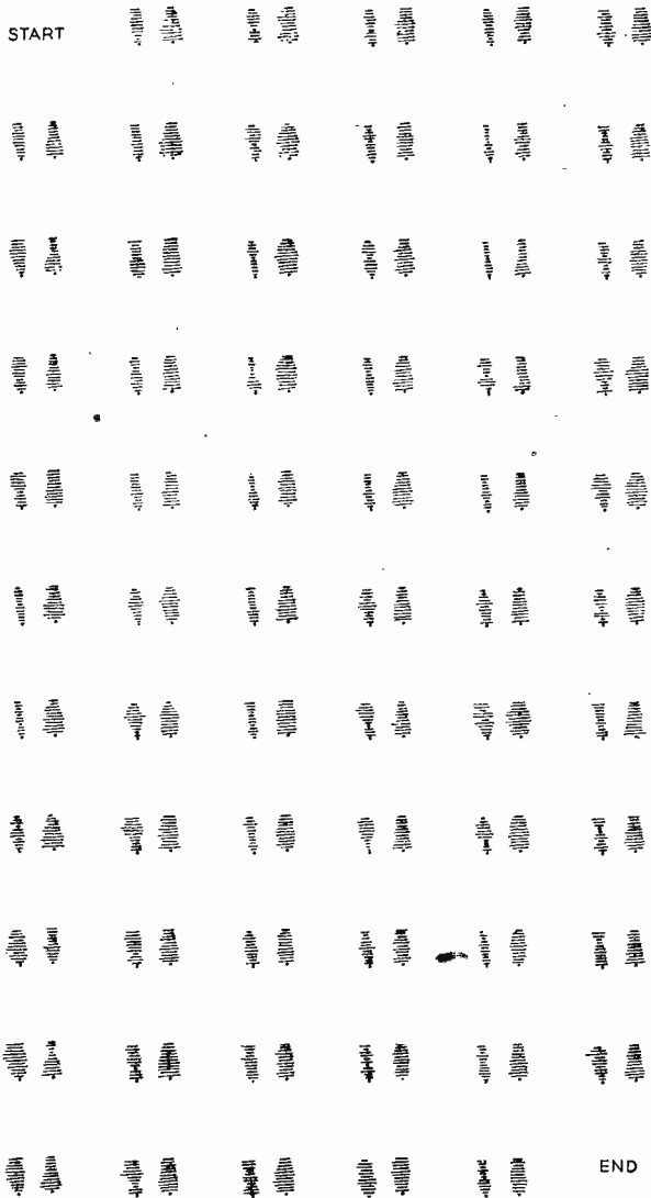
Fig. 27—This is a cathode-ray “multitone” record comparing the MUSA output with that of a horizontal half-wave antenna. The tones on the right-hand side of each frame are the MUSA output; those on the left are the output of the horizontal half-wave antenna. The two MUSA branches were steered at 15 and 22.5 degrees. A delay of 470 microseconds was used to equalize the transmission time. GCS (9020 kilocycles) Rugby, February 24, 1936, at 3:54 P.M. E.S.T.
