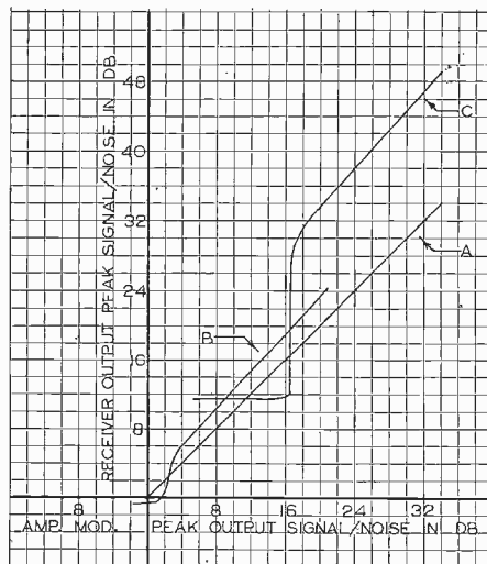
Fig. 15—Measured peak signal-noise ratio characteristics of impulse noise. Curve A = amplitude modulation receiver. Curve B = frequency modulation receiver with deviation ratio of unity. Curve C = frequency modulation receiver with deviation ratio of four.
