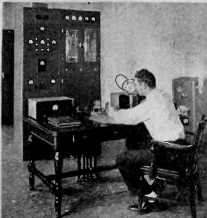
WESTERN ELECTRIC ultra high frequency Pollex Radio Transmitter, Station W2XEM, Newark, N. J.
