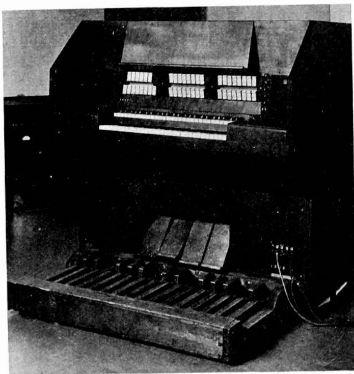
Fig. 10—Vierling-Kock organ using inductive neon tube circuits for tone current generation.
