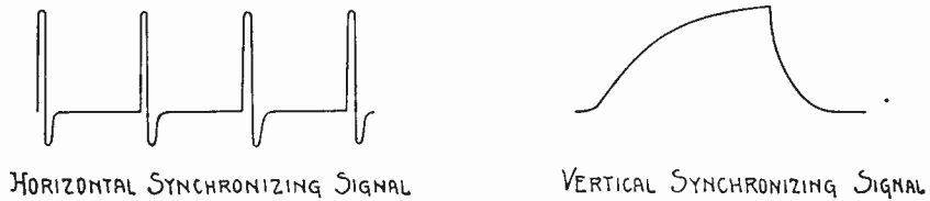
Fig. 13—Synchronizing signals after passing through separating circuit.
