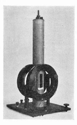
Fig. 1-Photograph of electrodynamometer.
