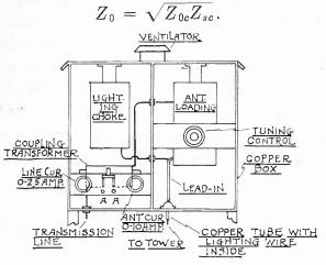
Fig. 15—Antenna tuning units.
