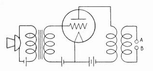
Fig. 3—Circuit diagram of vacuum tube to be used in place of resistance  $R_R$  of Fig. 1 to produce frequency modulation.
