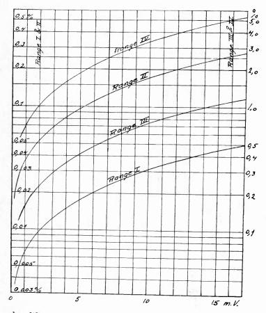
Fig. 21-Actual calibration curves for the four ranges of the ripple meter. The ordinates indicate per cent ripple modulation measured.
