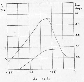
Fig. 2—Oscillating current and plate current shown as a function of the plate bias.
