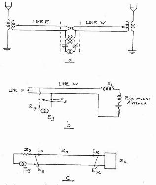
Fig. 3—Antenna excitation system and equivalent circuits. a. Actual circuit. b. Transformer replaced by leakage reactance. c. Final circuit analyzed.
