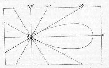
Fig. 3-Directional characteristics of the Yagi antenna.
