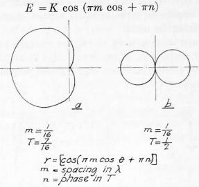
Fig. 1-Horizontal plane space patterns of two vertical antennas.
