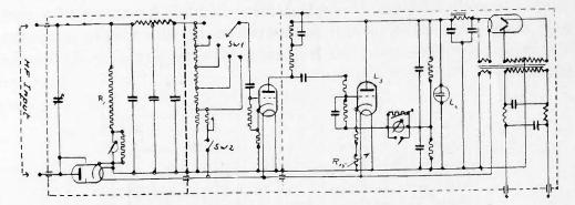
Fig. 19—Wiring diagram for a ripple meter used to measure exceedingly small degrees of ripple modulation.
