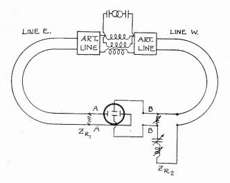
Fig. 8-Connection used for oscillograph tests.
