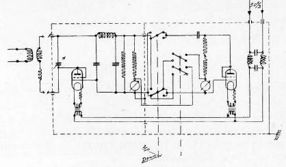
Fig. 17—Wiring diagram for the modulation meter.
