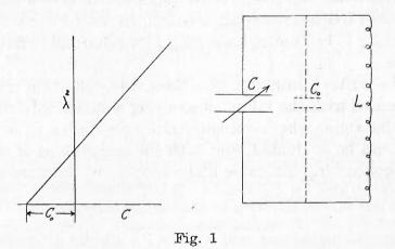
Lenz,<sup>1</sup> in his theoretical treatment of single-layer coils, determined the total charge of a single ring of an idealized coil. He took the coil as a capacity-free system to which were shunted such capacitances as would have the same effect as the charges actually on the coil. He found that the total coil capacity was one third as much as the ca-
