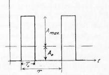
Fig. 2—Amplitude function illustrating a "sharp-dotted" modulation of a telegraph transmitter.
