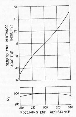
Fig. 2—Curves showing variation of sending end reactance and resistance with receiving end resistance.
