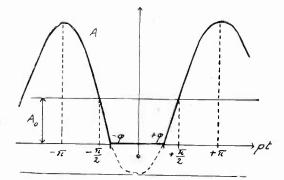
Fig. 6—Amplitude function illustrating overmodulation in a class C, high-frequency amplifier.
