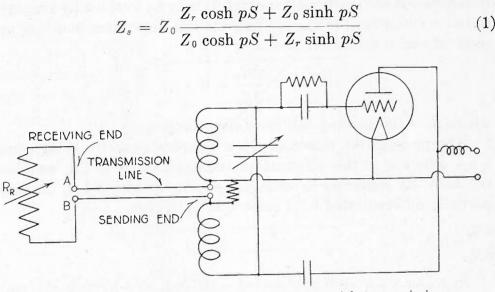
Fig. 1-Circuit diagram of Hartley oscillator with transmissionline modulator.
