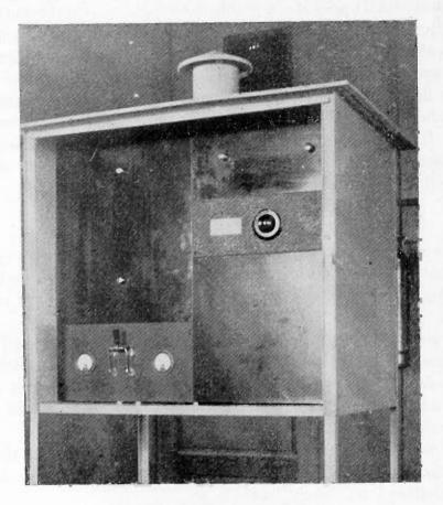
Fig. 16—Antenna tuning units.
