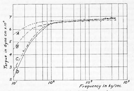
Fig. 4—Torque-frequency curves for disks of different conductances. Curves A, B, C, and D are respectively for silver disk No. 2, aluminum disk No. 2, zinc disk No. 1, and brass disk No. 1.  $H_v = 0.0731$  gauss.
