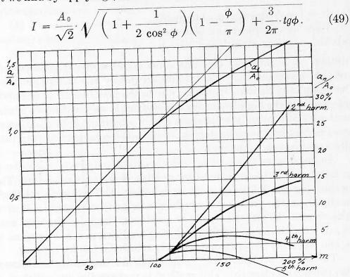
Fig. 8—Harmonic distortion spectrum showing Fourier components up to the fifth for overmodulating a class C amplifier.
