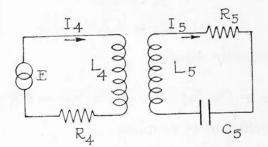
Fig. 4-Coupling transformer, equivalent circuit.
