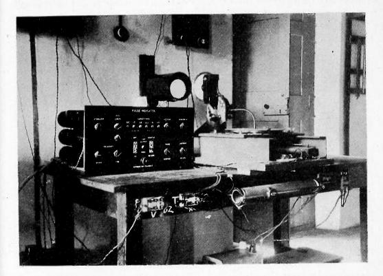
Fig. 6-Pulse indicator and recorder.
