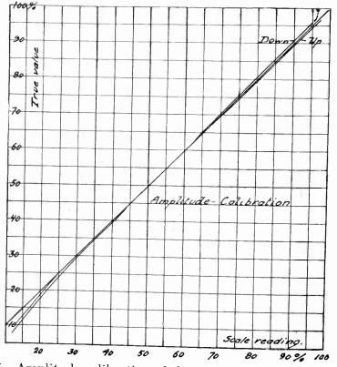
Fig. 15-Amplitude calibration of the described modulation meter.
