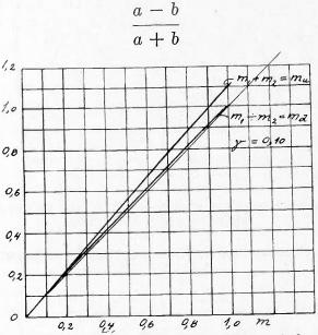
Fig. 5—"Up" and "down" modulations as functions of the degree of input modulation for  $\gamma = 0.1$  in a class B, high-frequency amplifier.
