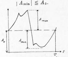
Fig.1—Illustration of an arbitrary but periodic amplitude function with the period T.
