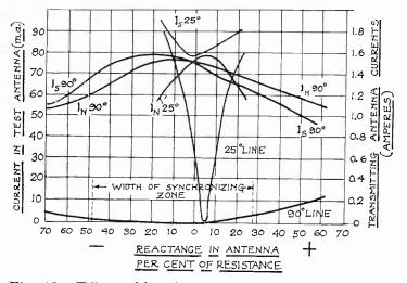
Fig. 13-Effect of low-loss lines on synchronization.
