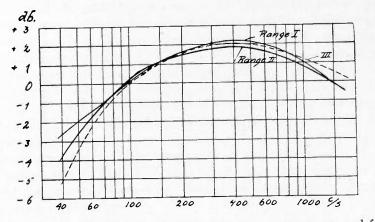
Fig. 22-Frequency responce of the ripple meter, measured for the ranges I, II, and III.
