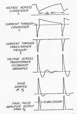
Fig. 2-Voltages and currents in various parts of the pulse generator.
