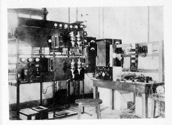
Fig. 4—Transmitter and pulse generator with cathode ray oscillograph monitor.
