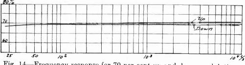
Fig. 14—Frequency response for 70 per cent up and down modulation by use of the filter finally adopted.
