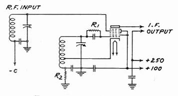
Fig. 5-Noninterlocking circuit.
