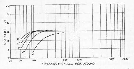
ig. 2—Low-frequency response of an electrodynamic cone speaker with 48- by 48-inch baffle showing effect of diaphragms of from 4- to 12-inch diameters upon the low-frequency cut-off.
