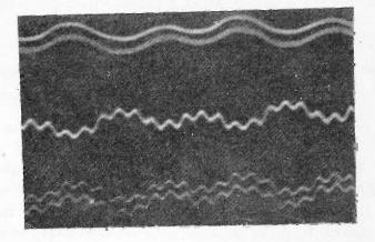
Fig. 12—Oscillograms of modulating and demodulated waves. The carrier was 75 megacycles. The smooth oscillograms at the top are the modulating wave (above) composed of 100 and 200 cycles with the demodulated wave below. The two waves at the bottom are the same as those at the top with 1000 cycles in addition. The center shows the two lower waves superposed.
