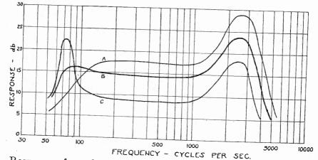
Fig. 3—Response of an electrodynamic cone speaker at various gap densities. Curve  $\hat{A}$  is with gap density of 9600 gausses, curve B is with 7000 gausses, curve C is with 3500 gausses.
