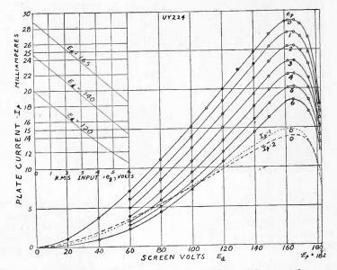
Fig. 10—Transrectification characteristics of two tubes with  $e_{\sigma}$  in volts rootmean-square. The broken lines are the static characteristics for the separate tubes; their ordinates when added give the  $e_{\sigma} = 0$  curve for the two tubes.
