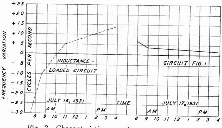
Fig. 2—Characteristic operation—790 kilocycles.
