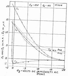
Fig. 3—Solid lines: static characteristics; broken lines: peak and root-meansquare transrectification characteristics.
