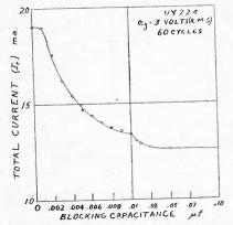
Fig. 7— $I_i$  as a function of blocking capacitance at 3 volts input.
