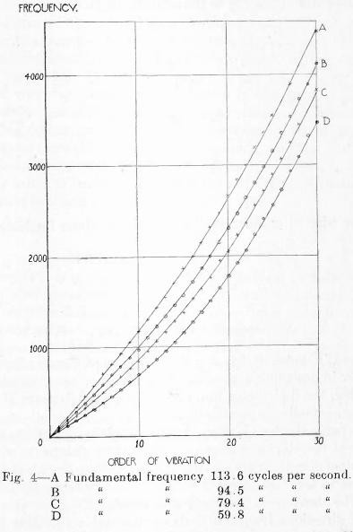
an error of only 1.7 per cent in that of the twentieth mode. The curves shown in Fig. 4 are the curves of frequency calculated from (5) using
