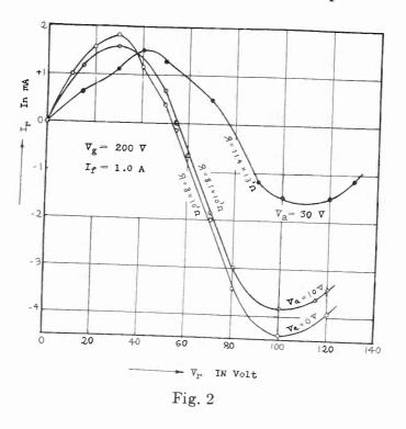
primary electrons may not have sufficient energy to cause secondary emission when they impinge upon the surface of the inner grid.
