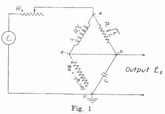
If we desire a stable tuned resonant circuit for purposes of tuned radio-frequency amplification instead of a self-oscillatory circuit, we may obtain it by increasing the value of the negative dynatron resistance  $-R_p$  fractionally. Let this fractional increase be -R ohms a quantity small compared to  $-R_p$ . This resistance R will then act to prevent self-oscillation and determine the "decrement" in the same manner as in the reactance tuned circuit.
