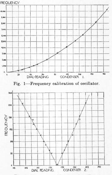
Fig. 2-Frequency calibration of oscillator.
