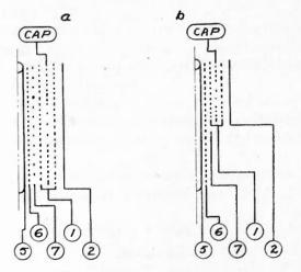
Fig 9—Proposed form for tube structure. a. Existing form of 2 A 7 b. Proposed change
