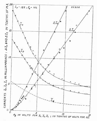
Fig. 6—Transrectification characteristics. On the  $I_p$  and  $I_t$  curves the small circles are points taken at 60 cycles, the crosses at 750 kilocycles. On the  $\Delta I_p$  and  $\Delta I_t$  curves the circles are at 60 cycles, the solid dots at 750 kilocycles.
