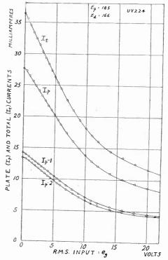
Fig. 11—Transrectification characteristics;  $I_p$  and  $I_t$  for two tubes; the curves  $I_p - 1$  and  $I_g - 2$  are the individual curves which when combined give the  $I_p$  curve.
