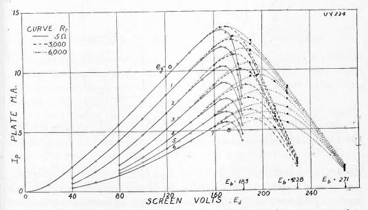
Fig. 5—Transrectification characteristics with indicated load resistance in plate circuit.  $e_q$  in volts root-mean-square.
