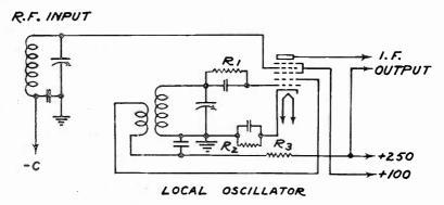
Fig. 1-Conventional pentagrid converter circuit.
