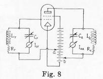
If we connect parallel resonant circuits in the inner grid and the anode sides as shown in Fig. 8, two oscillations having their respective resonant frequencies will be maintained, provided the various elec-
