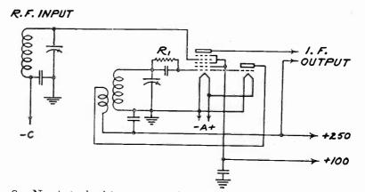
Fig. 8-Noninterlocking circuit for tubes with filament cathodes.
