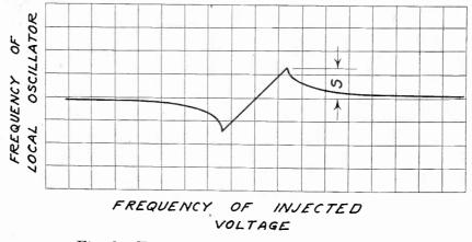
Fig. 2-Typical interlocking characteristic.
