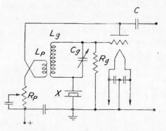
Fig. 1-Oscillator circuit.
