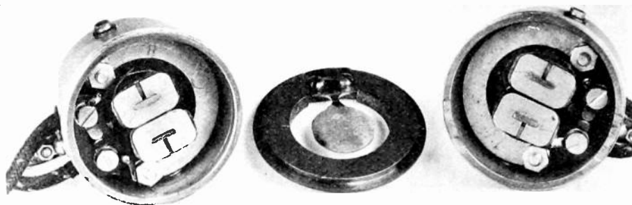
Fig. 1—Exploded view, showing tuned reed, motor, and generator units.
